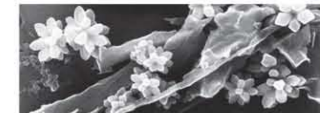
Not an apple blossom, but an aluminum alloy: quasicrystal's 5-fold symmetry conveys a strange life-like quality
